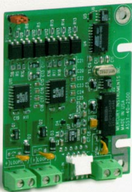
New Mercury 4-to-20 milliamp output board.
