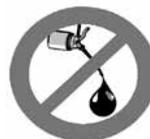
**IMPORTANT: DO NOT** add oil to the permanently lubricated Series 3 Accessory Unit.
